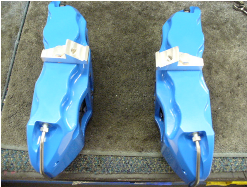
Hose adaptors installed to allow use of original hoses.
