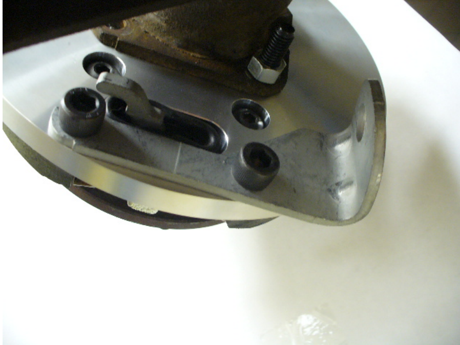
Park assembly installed on drivers side
