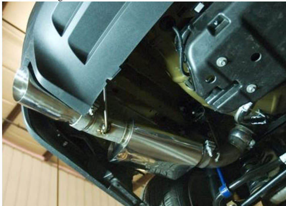
Figure 1: Installation of DS Muffler Assembly
