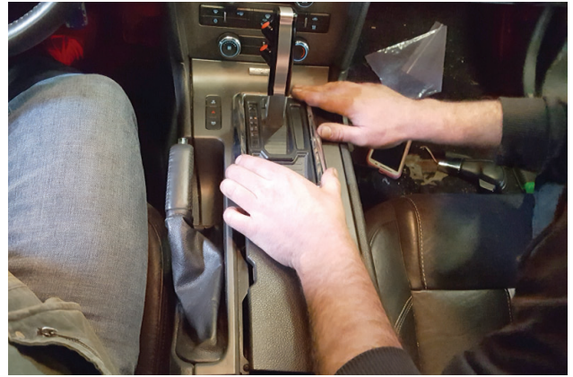
15. Press console down into place then replace shifter trim (removed step 2).
