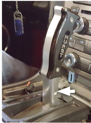
13. Install (x2) screws (9) to secure shifter in place.
