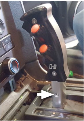
13. Install (x2) screws (9) to secure shifter in place.
