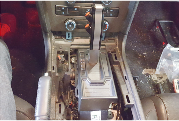
12. Fit top of shifter down into place, securing (x4) tabs around its side (disconnected step 8).
