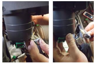
4. Unplug connectors and detach connector from bottom of console.
