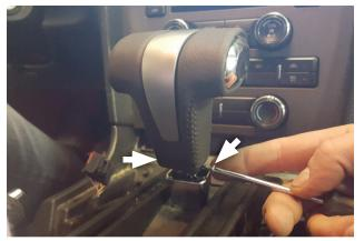
6. Separate bottom of shifter knob being careful not to scratch it. Remove (x2) screws securing both sides of shifter knob to stem.
