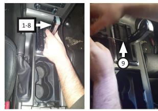
12. Install assembled **shifter (1-8)** and secure it in place with (x2) **screws (9)** as shown.
