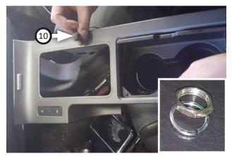
9. Choose install location (somewhere that wiring reaches shifter) then drill a <sup>1</sup>/<sub>32</sub>" hole. Remove nut and lock washer from assembly, then pull switch wiring through hole until button is flush with console wall. Use nut and lock washer to secure button in place.
