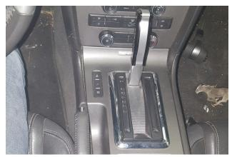
13. Press console down into place then replace shifter trim (removed step 2).
