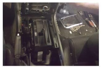
8. Remove shifter handle from stem then remove shifter plate.
