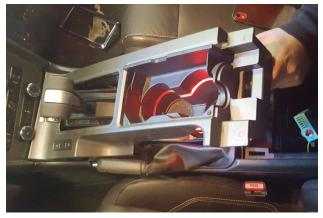
3. Lift console from rear to disconnect it from tabs securing it down.
